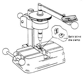
FIG. 2 Torque-Measuring Device
