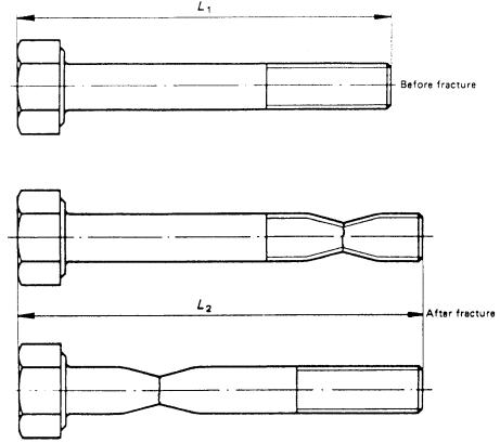
FIG. 1 Test Specimen-Extension Test
